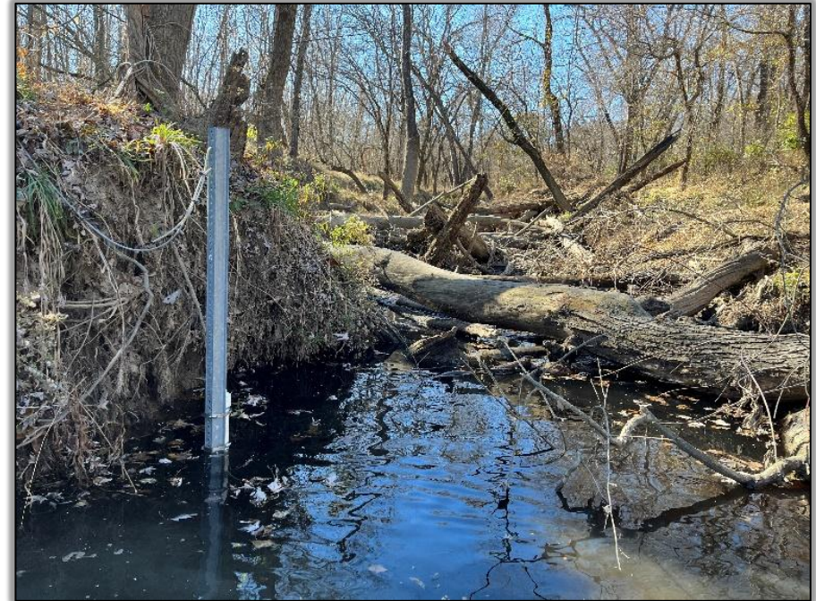
Post mount monitoring station, Mill Creek
