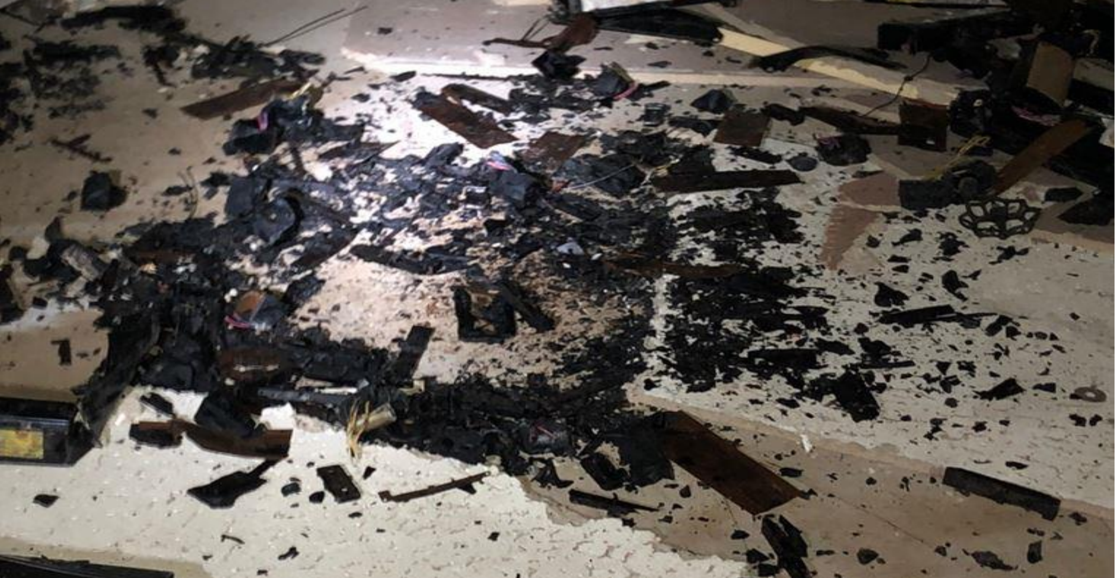
Potting Material (Tar/Asphalt/Resin) Black, sticky material that surrounds internal parts.
